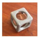
Create a ship-in-a-bottle-esque coin cube for a penny. Use variables to create a cube that is quickly customizable for a coin of any radius.
